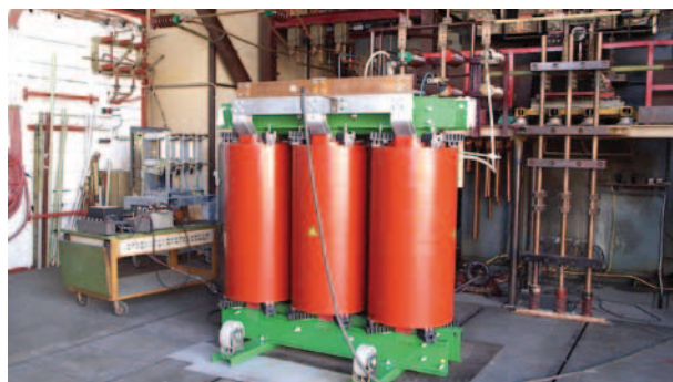
Short circuit test at CESI (MI)
