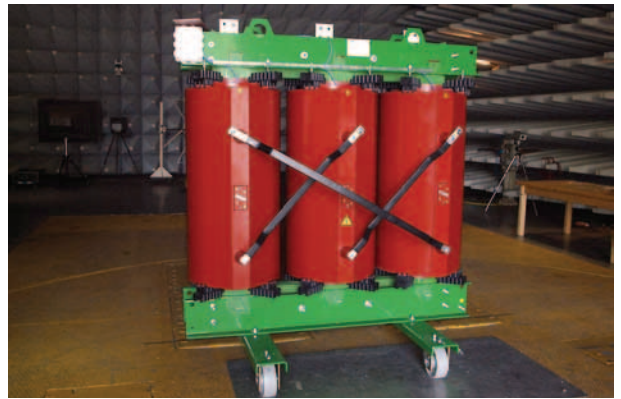
One of our transformer during the measurement of sound level at CESI (MI)
